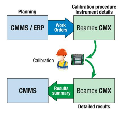
Typically, work is planned, and work orders are created in the maintenance management system. With an integrated solution, these work orders move automatically and digitally from the maintenance management system to the calibration software. There is no need to print work orders and distribute them manually.
