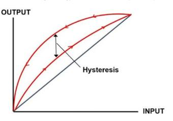
the span and test points back down the span. Critical in this approach is that the technician not overshoot the test point and reverse the source signal, approaching the test point from the wrong direction. Technicians should be instructed to return to previous test point and approach the target point from the proper direction.
