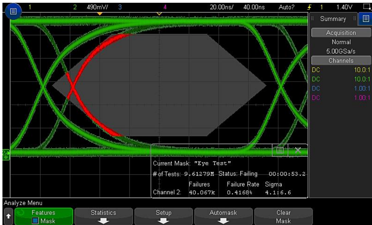
Figure 27. Hardware accelerated mask testing allows testing against a golden waveform or user created mask to find violations. In this example we captured over 5M tests in only 30 seconds.
