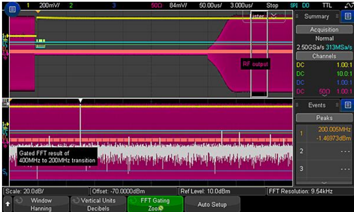
Figure 21d. RF signal settled down at 200 MH as indicated in the search lister.
