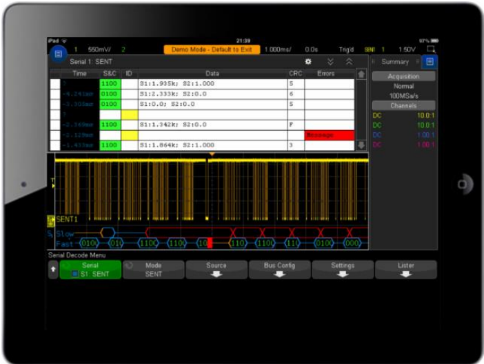
Figure 8. Remotely control the 3000T X-Series via tablet device.
