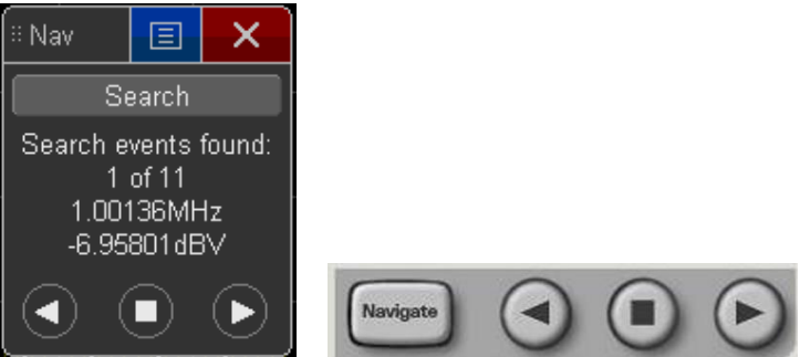
Close-up on buttons on the front panel of the scope. Alternatively, you also can use the touch navigation control.
