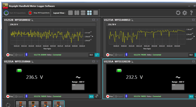
Figure 13. View up to 10 handheld meters readings or trendings with Keysight Handheld Meter Logger software
