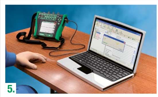
Upload the results from a calibrator/mobile device to CMX software.
